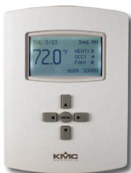
BAC-120163CEW (Optional Humidity Sensor, 6 Relays, 3 Analog Outputs, Optional Ethernet/IP Communication, White)
