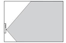
The effective detection range is approximately 10 meters or 33 feet. Factors that may reduce the range include:
