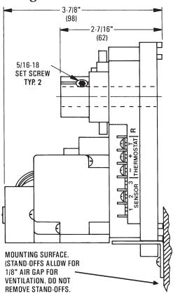
These controller-actuators are designed to mount on a standard 1/2 in. (13 mm) diameter shaft or a 3/8 in. (9.5 mm) shaft using the optional HFO-0011 adaptor.
