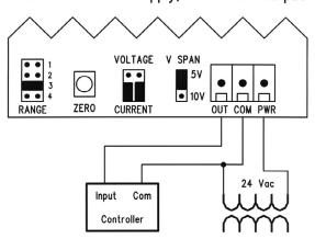
24 Vdc Power Supply, 4-20 mA Output
