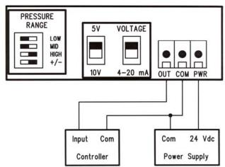
24 VAC Power Supply with 4-20 mA Output
