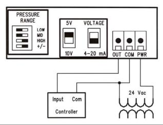
24 VDC Power Supply with 4-20 mA Output
