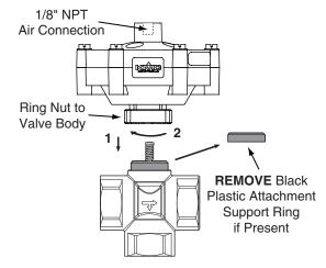
**Mounting Actuator on Valve Body**
