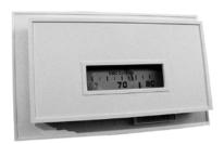
The CTE-1001/1002 electronic thermostats are designed for use with specific CEE/CEP/CSE/CSP-4000 series controller-actuators for controlling damper actuators and/or valves in HVAC systems. The ability to adjust minimum and maximum limits is at the thermostat rather than at the controller. They are single setpoint units for cooling and heating applications. Several mounting methods are available.
